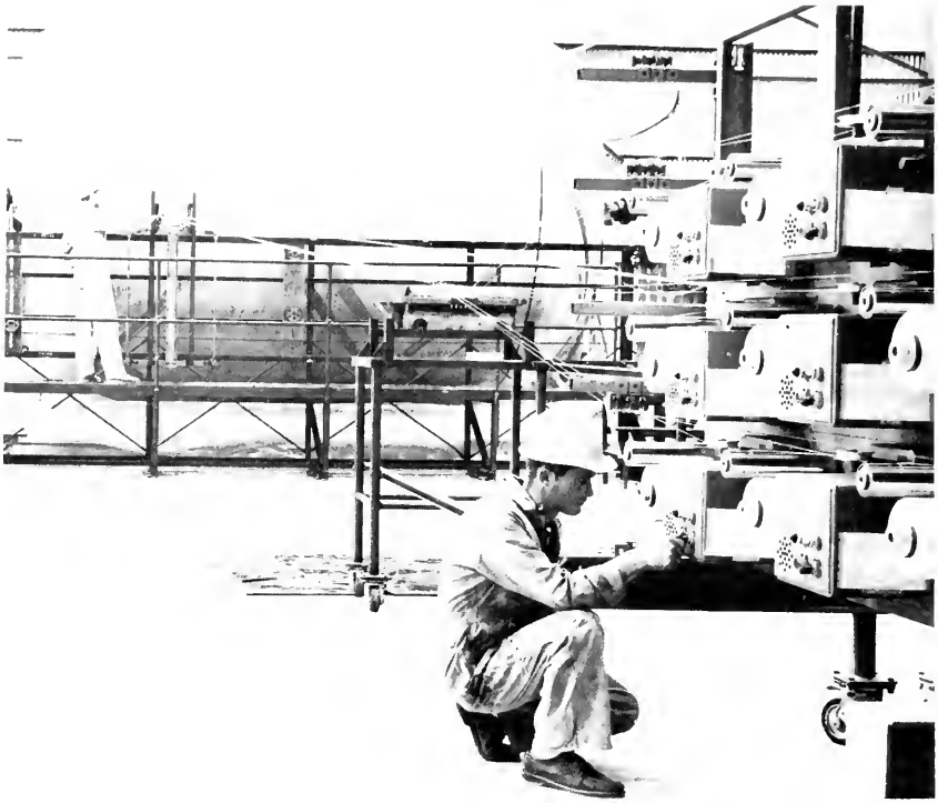
FIGURE 8-8.—A solid-propellant rocket-motor case segment being wound with glass-fiber filament. (Courtesy of United Technology Center.)
